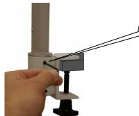
Tighten the upper grub screw (M6x6) so that the foot of the support arm presses firmly against the clamping device.
